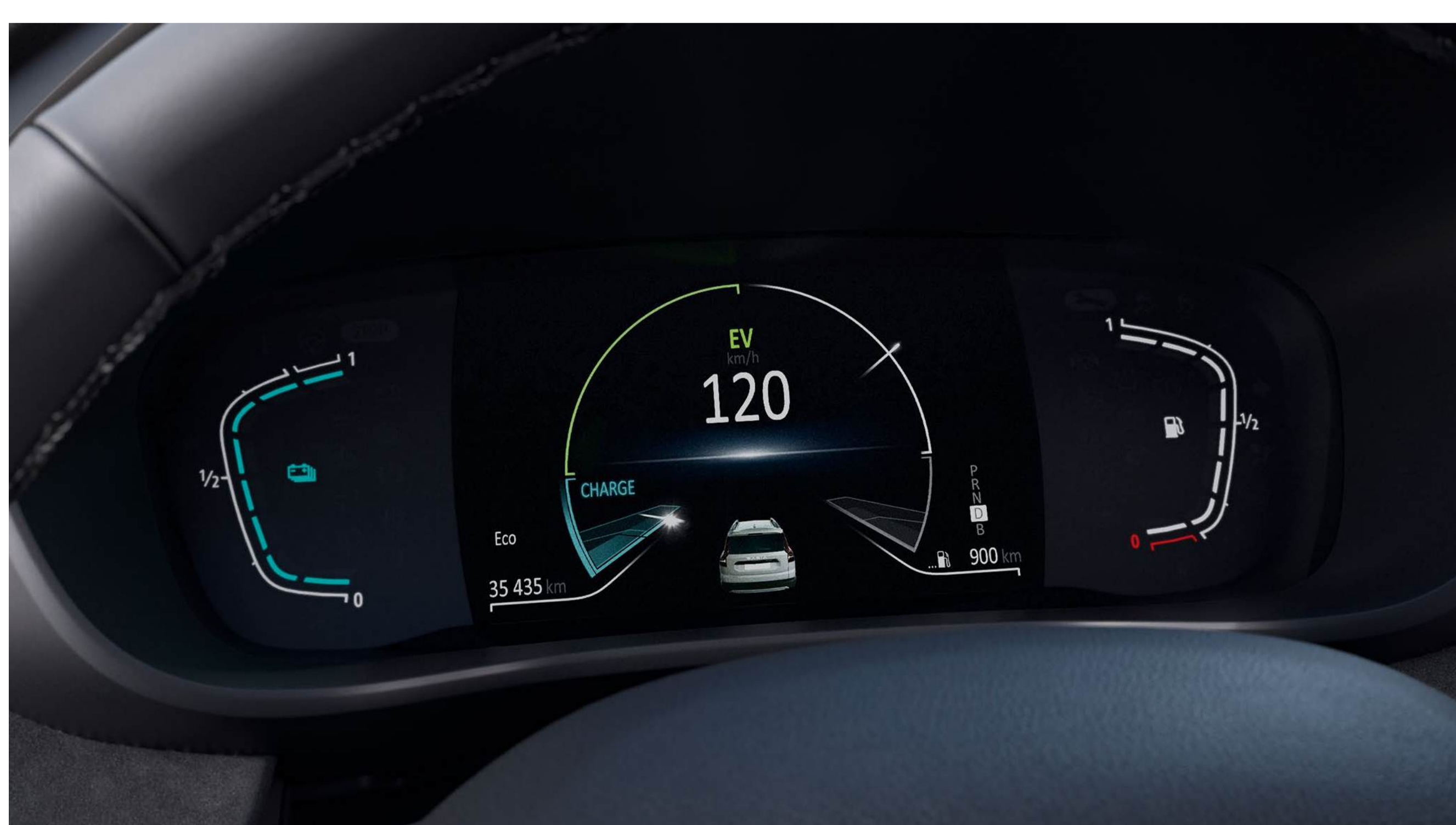
7" Colour cluster with driving mode information
